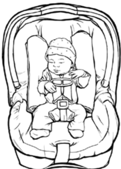
Figure 2: Car safety seat with a small cloth between crotch strap and infant, retainer clip positioned at the midpoint of the infant's chest, and blanket rolls on both sides of the infant.
